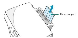
**2** Fan the paper and insert it with the print side facing you. Ensure that the right edge of the paper is in contact with the right side of the paper bin. Do not exceed the specified capacity.
